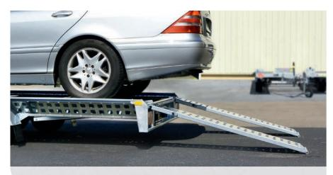
Loading ramps retain contact with the ground during tipping.
