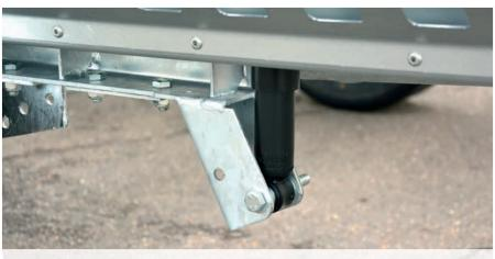
Dumping body can be tilted with dampers (maintenance free, hydraulic)
