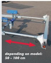
useful: extendable loading area through retractable and removable light rail.
