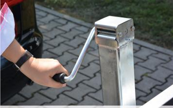
By pressing the telescopic crank the tipper bridge is brought into the desired position.
