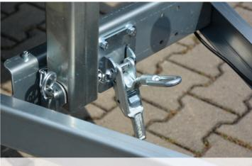
Attachment of the tipper bridge using safety release fastener.
