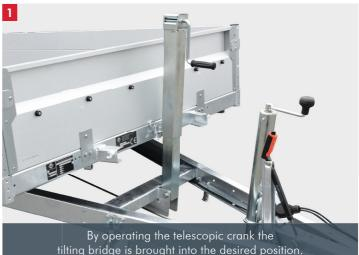
tilting bridge is brought into the desired position.
